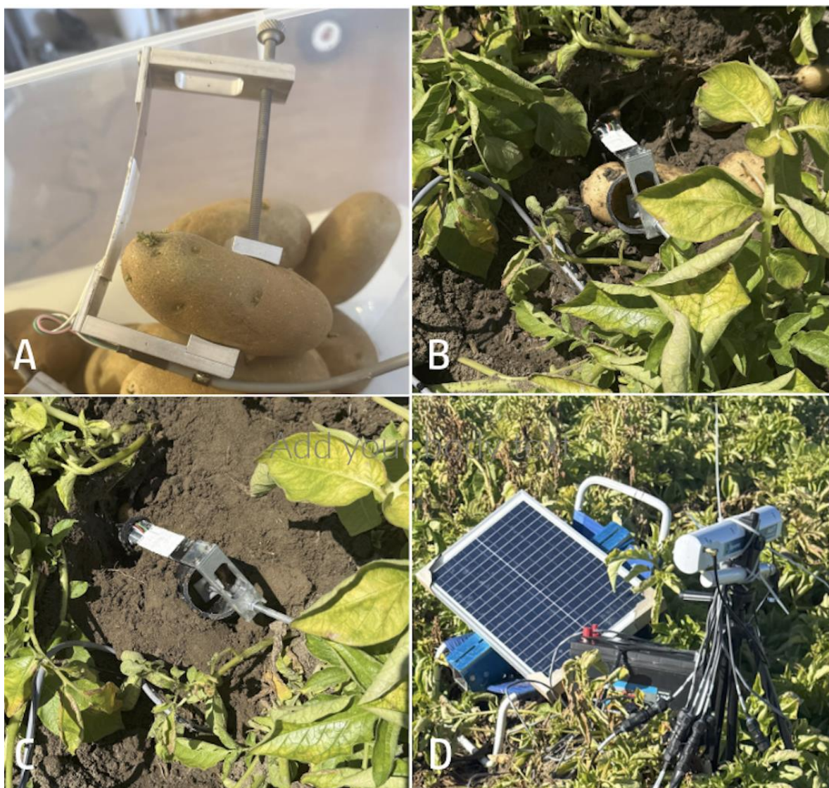
Figure 1. Tuber sensor and field implementation. (A) The strain gauge C-clamp [7] model DEX100 (Dynamax Inc., Houston, TX, USA) on a potato tuber. (B) The sensor was placed on the cleaned upper surface of the tuber. The metal anvil contacts the cleaned tuber and is inserted through an approximately 3 cm-long black plastic pipe, flush with the tuber surface, pointing north. (C) The sensor on the buried tuber, except where the soil was blocked by the black plastic pipe. The square metal anvil is touching the potato inside the pipe, as shown in Figure 1A, and is positioned to measure the height dimension. (D) The equipment (Dynamax, Inc.) set up on July 9 included a solar panel, a 12-volt deep-cycle battery, an air temperature sensor inside the white data logger housing, and a data logger with a transmitter mounted on a tripod.
